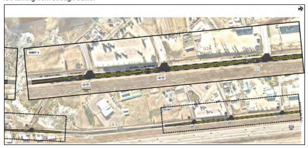
FIGURE 10 - CONCEPT #1 - NEW LEFT-TURN LANES ALONG SALT CREEK HIGHWAY,
